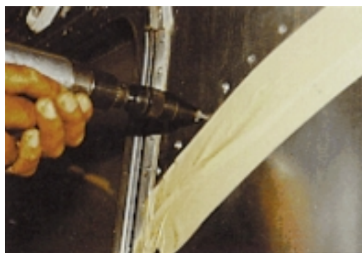
2. PROPER SIZED SHAVER TOOL, INSTALLED IN A STANDARD 1/4" DRILL, SHAVES RIVET HEAD.
