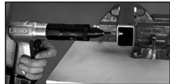
Depress the lower trigger and the tool unthreads from the installed part.
