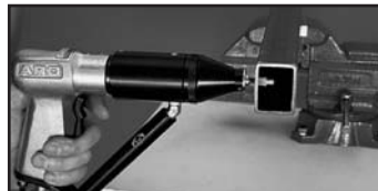
1/4 turn the fastener onto the SPP tool mandrel and place the fastener into the hole.
