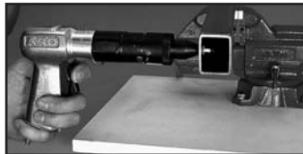
Depress the top trigger until the tool stalls and the AVK fastener is collapsed.
