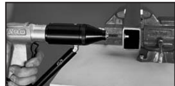
Depress the tool reverse trigger and the tool spins out of the installed fastener.
