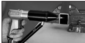
Depress the tool trigger and the tool spins into the fastener and automatically exerts a pressure controlled pull installing the fastener.
